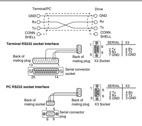
Figure 3-11. X3 D-type Connector RS232 Connections
